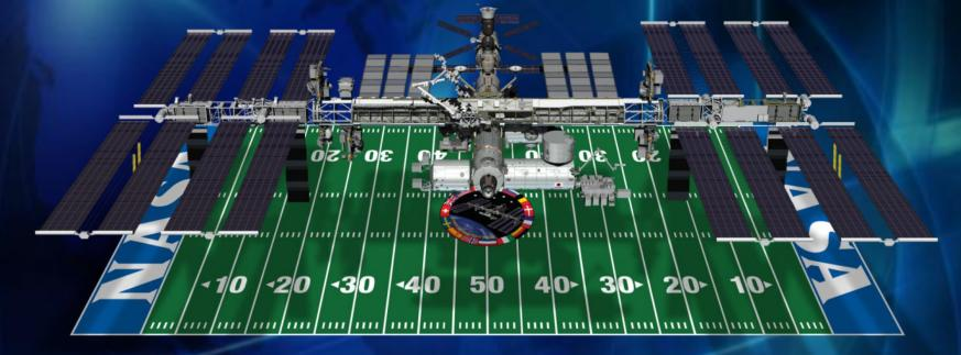
Spacecraft Mass: ~925,000 lb (~419,000 kg) Spacecraft Pressurized Volume: 32,333 ft3 (915 m<sup>3</sup>) Velocity: 17,500 mph (28,200 kph) Altitude: ~220 miles above Earth Power: 80 kW continuous Science Capability: Laboratories built by US, Europe, Japan, and Russia Extended through *at least* 2020
