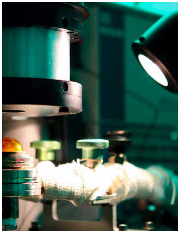
Diffuse Reflectance Infrared Fourier Transform Spectroscopy is a technique that allows researchers to investigate the chemical reactions that occur on the surfaces of catalysts. (Photo courtesy Oak Ridge National Laboratory/ Photo by Jason Richards.)
