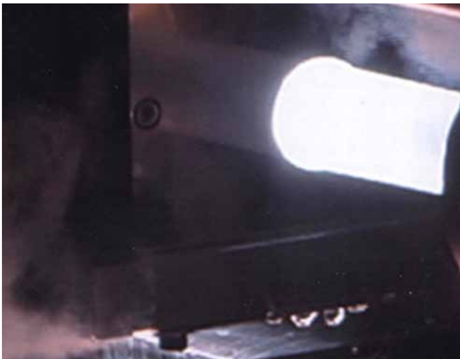
High-density infrared transient liquid coating process (Photo courtesy of Courtesy: Oak Ridge National Laboratory)
