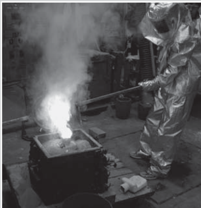
Figure 1. Fank pours bronze into an investment mold at UW-Madison's Spring 2007 Engineering Expo. The event helped to renew interest in the university's foundry, which had been shut down in the 1990s.
